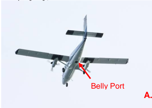
Figure I-4. A) The NOAA Twin Otter (N57RF) with open belly port. B) The three Canon EOS-1DS Mark III cameras with 85 mm lens housed in the FMC mount.
