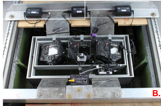
Figure I-4. A) The NOAA Twin Otter (N57RF) with open belly port. B) The three Canon EOS-1DS Mark III cameras with 85 mm lens housed in the FMC mount.
